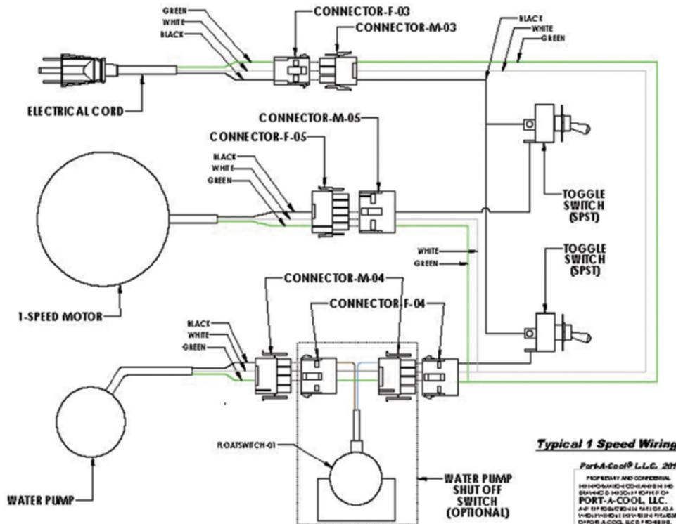
**Typical 1 Speed Wiring**
