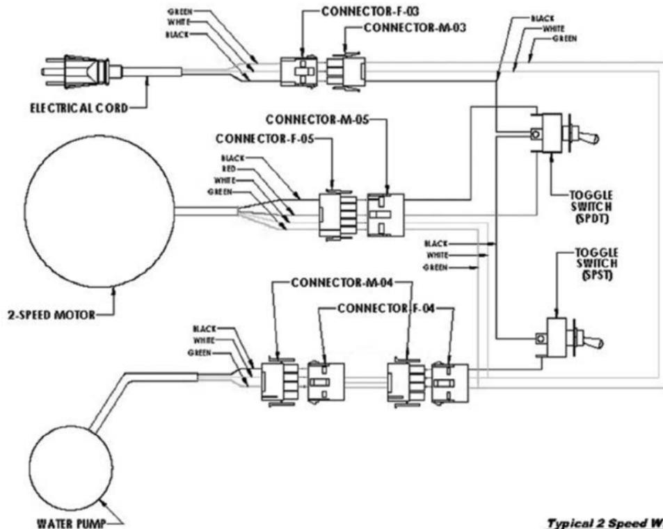
*Typical 2 Speed Wiring*
